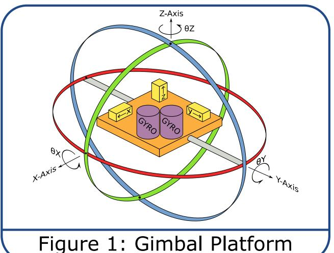
Measuring linear acceleration is straightforward, but measuring the angular acceleration is more difficult. In the past, a gyroscope-stabilized gimbal platform was used (see Figure 1), but this is a heavy mechanical device and has problems with maintainence and wear, as well as weight and expense. Micro-electromechanical systems (MEMS) gyrometers are very expensive, especially when compared to MEMS accelerometers.
