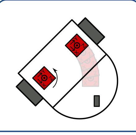
Figure 4: Rotation with 2 Accel. We can further extend this idea to all three dimensions by adding a third accelerometer unit. If we ensure that all three sensors are not colinear, then we will always be able to detect any vehicle rotations.
